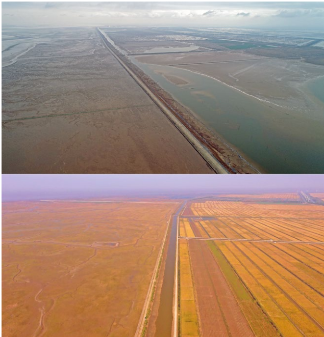
FIGURE 2 An aerial view of the current seawall at Tiaozini of southern Jiangsu Province (upper panel) and Chongming Dongtan (lower panel) of Shanghai, China. The seawall breaks the bare (upper panel) or vegetated (lower panel) upper tidal flat away from the natural intertidal wetlands (left of the seawall) and converts the natural tidal flats into aquaculture ponds and arable land (right of the seawall) (Photographs provided by Chia-Yang Tsai and Shunqi Bo)
